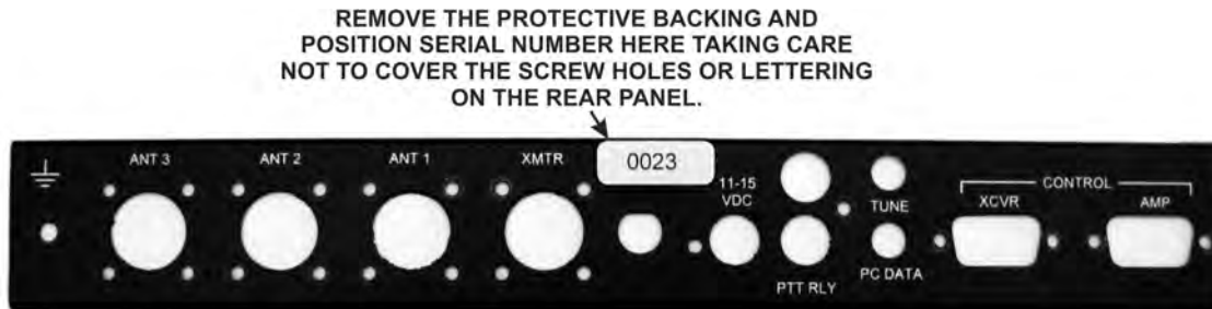
Figure 19. Attaching Serial Number to Rear Panel.
