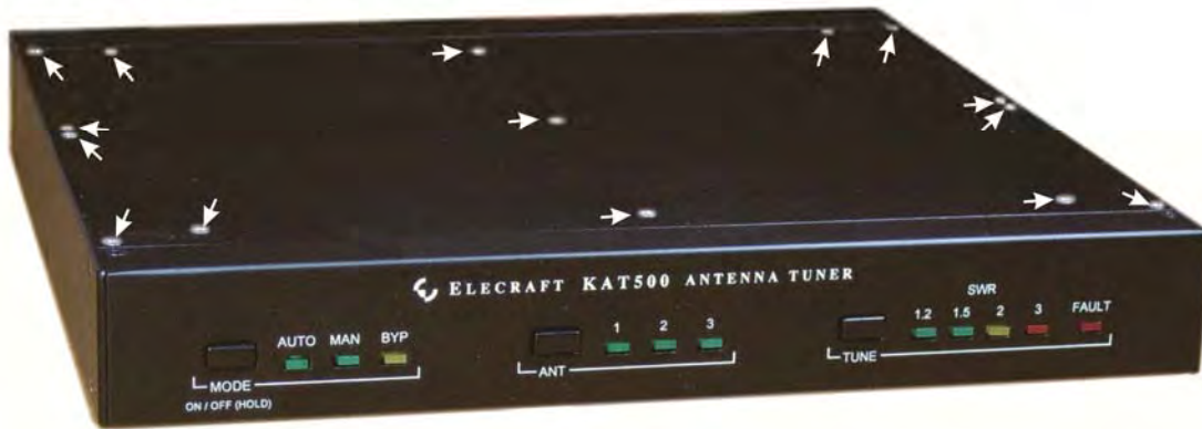
Figure 36. Installing the Top Cover.
