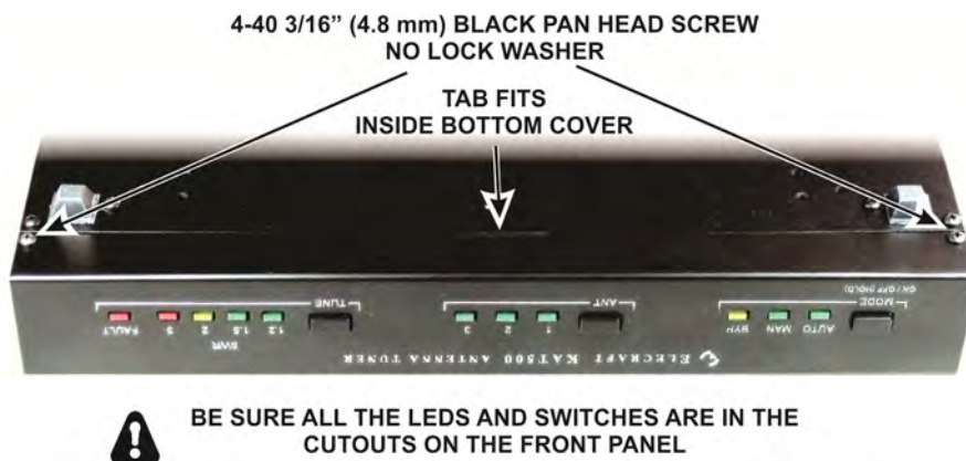
Figure 32. Mounting the Front Panel.
